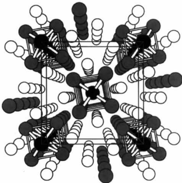
Fig. 1. An (001) perspective projection of Ta 5 Sb 4 . Light circles are Sb atoms and dark circles are Ta atoms.
